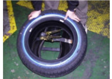
11. The tire can be turned over and a tire spoon may (carefully) be used to help push the tooth of the runflat further into the tire cavity. It is important not to use so much force that you cut the tire bead or deform the tire bead wire. Please note you must have at least 60 to 70% of the runflat in the tire or it will not install.
