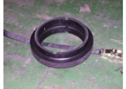
5. Feed strap end through slot in hub barrel and pull the strap tight against Runflat. Place the belt just slightly off center of the runflat. (approximately 60/40)
