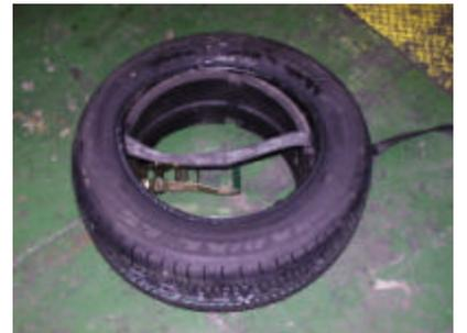
13. Remove the ratchet and strap assembly and align the runflat device with the beads as shown in the adjacent picture.
