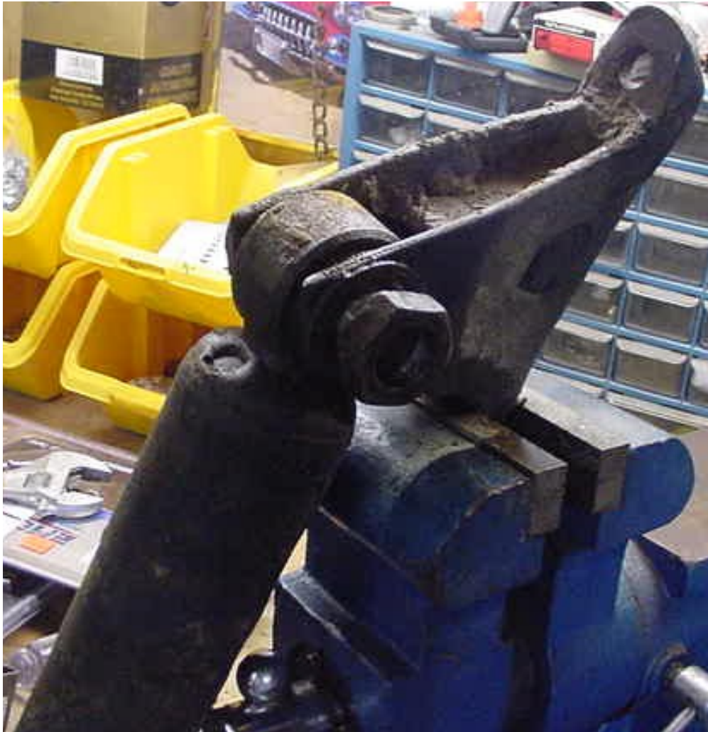
Shock in vice with lower bolt loose
