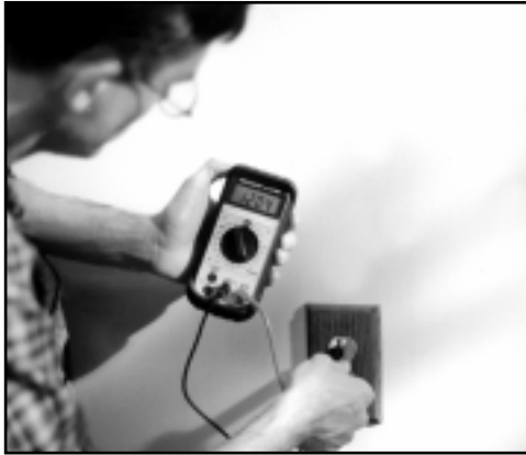
Measuring the voltage of a standard residential outlet is one example of testing AC voltage.
