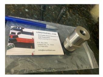
11. Install a 6.5L Diesel Head Cooling Kit. You really shouldn't see a "head cooling kit" on this thread because it doesn't add any cooling capacity, it does however circulate coolant to the rear of the engine water jacket to make cooling more even over the
