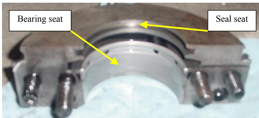
Rear Main Bearing Cap (seal removed)
