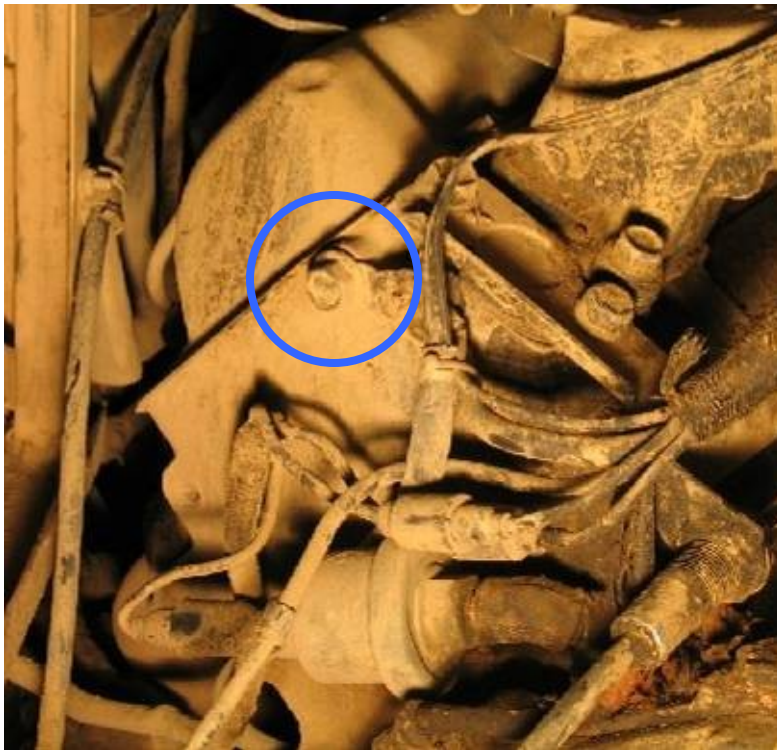
Main Engine ground – Left rear cylinder head (might be right side depending on model)
