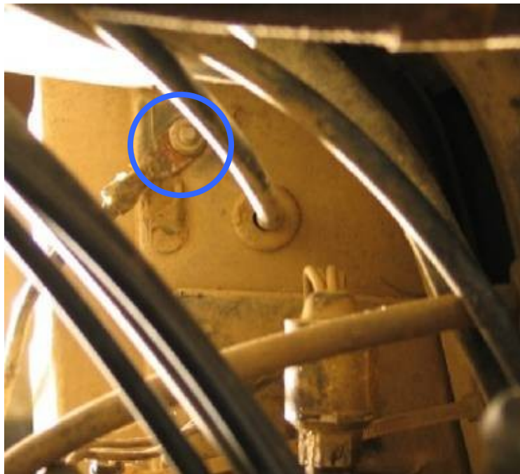
Engine side, Main Body Ground – Located above fuel filter
