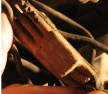
Picture of the electrical junction in the Humvee wire harness
