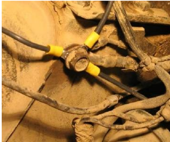
New Connections at the Engine Ground
