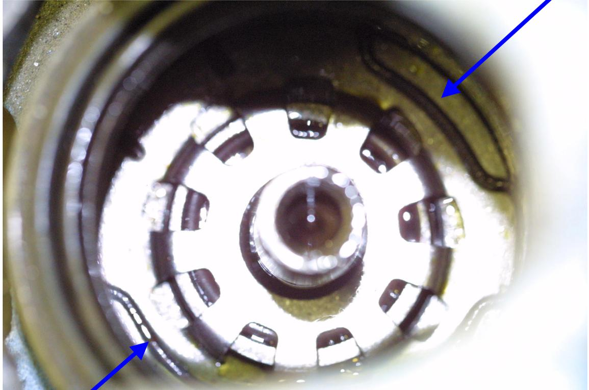
With long needle nose pliers, compress here, then place the SK hooks under the spring.
