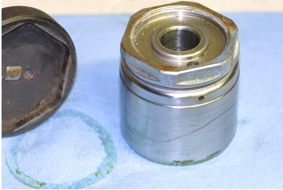
6. Once the piston has been freed from its seat on the thrust screw, pull it out of the dust boot.
