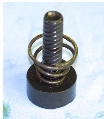
10. With the thrust screw removed, remove the thrust screw centering pin plug, spaced and finally with your finger inside the piston cylinder push the centering pin out. Discard O-ring.
