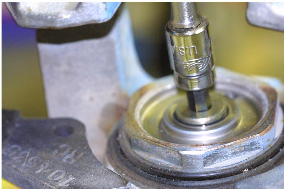
5. To remove the piston, I used the Breggin tool with a 3/8 extension and ratchet. <http://www.bluehammer.com/rebrcacoto.html> You then turn the piston counterclockwise. This can remove the piston about 2/3 of the total distance quickly. Then, you must remove this tool and use large channel locks on the same flat surface to totally unscrew the piston. Protect the surface from scratching.
