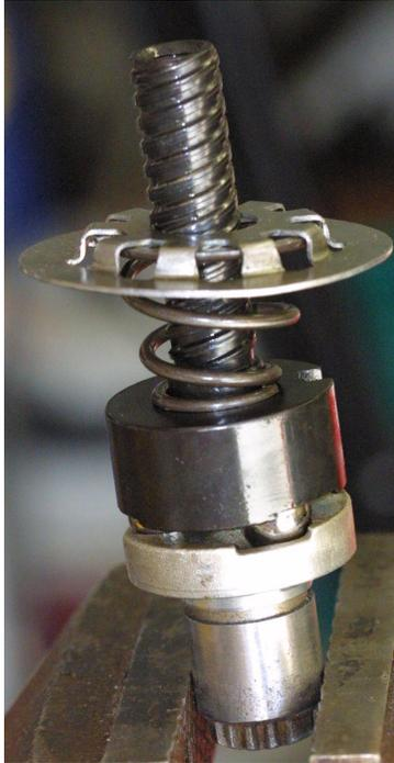
The thrust screw and the actuator shaft have between them three steel balls. These balls fit into eccentric indents. This will provide a one-way movement to the thrust screw when under compression. This is why when changing brake pads you must both compress and rotate the piston to retract it.
