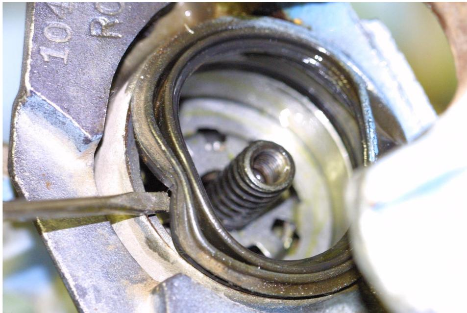
8. To remove the thrust screw-retaining ring (spring), it is easiest if you have the correct tools. I would recommend using the **SK HAND TOOLS - HOOK & PICK SET, 90353**. Either be very careful to not touch the inner piston cylinder surface or wrap the tools with a thin layer of electrical
