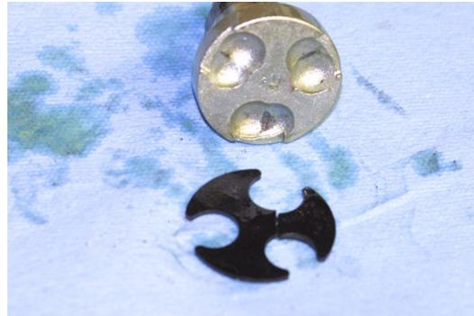
13. Pry off the actuator shaft dust seal and discard.
