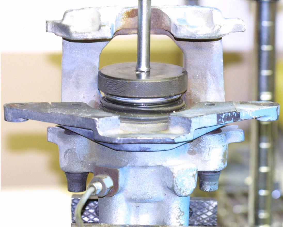
The Breggin tool fits on top of the piston that has a hexagonal surface prior to the actual smooth surface of the piston cylinder itself. You should carefully wrap or protect the piston surface to prevent any scratches that can lead to fluid leaks later.
