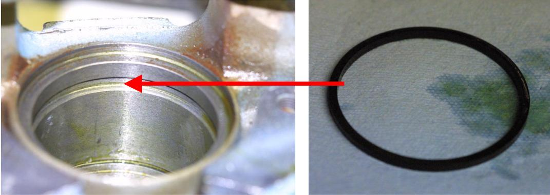
15. In my opinion, there is no purpose in disassembling the caliper piston since in my modification of the reassembly procedure we will reassemble the mechanism without the aid of the piston being used to push the thrust plate and thrust plate ring into position (the AMG recommended procedure)
