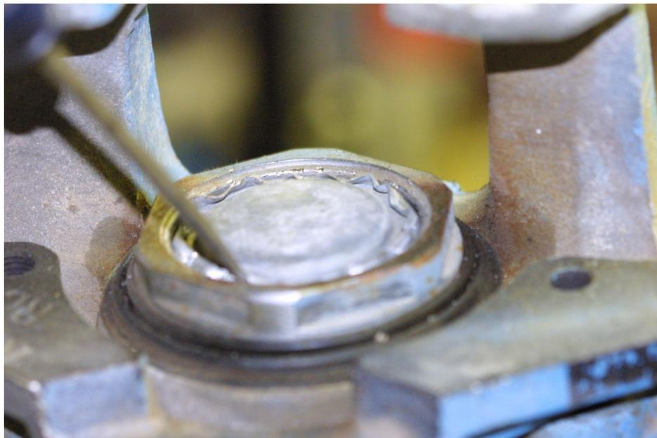
4. Remove the piston retaining screw with a hex socket. This screw has a rubber O-ring seal and a beveled shaped.
