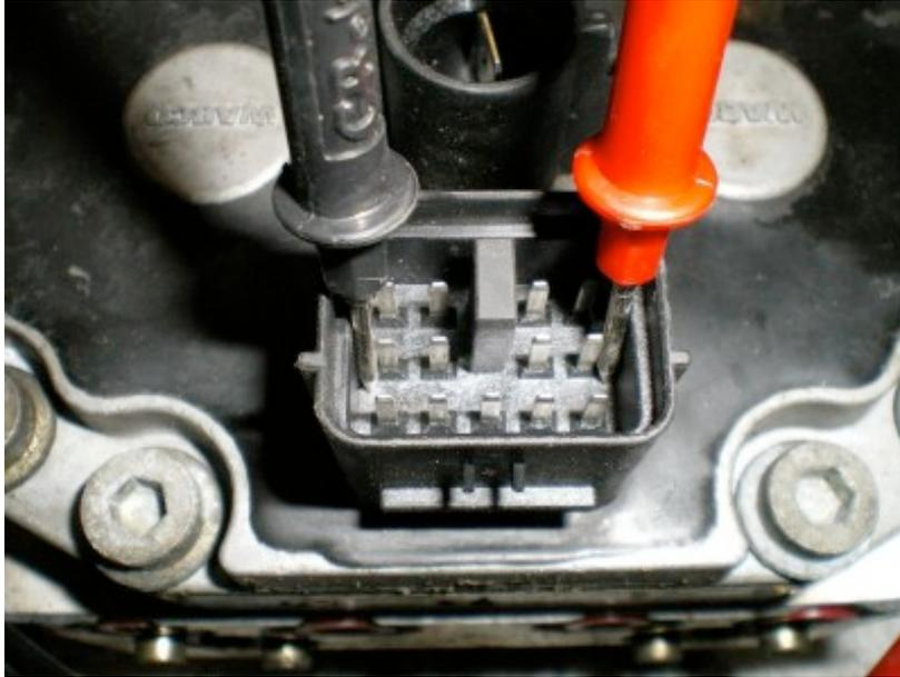
This is part of AM General's test procedure that verifies that the shuttle valve is bad, except you can do theirs directly at the ABS ECU connector (pins 25 and 27). Okay so back on track this gave me no connection between pin 6 and 9. The shuttle valve is located on the bottom of the modulator, it's a piece of black plastic that runs the span of the modulator and is held in with three Allen head screws.
