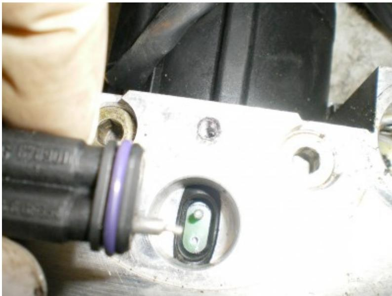
Here's some insight into how the shuttle valve works, the plungers are activated by two different diameter plungers located within the modulator. The more pressure you put on the brake pedal, it activates the two different plungers accordingly. That is how your vehicle knows if your not braking, lightly braking, or to the floor "oh crap" braking.
