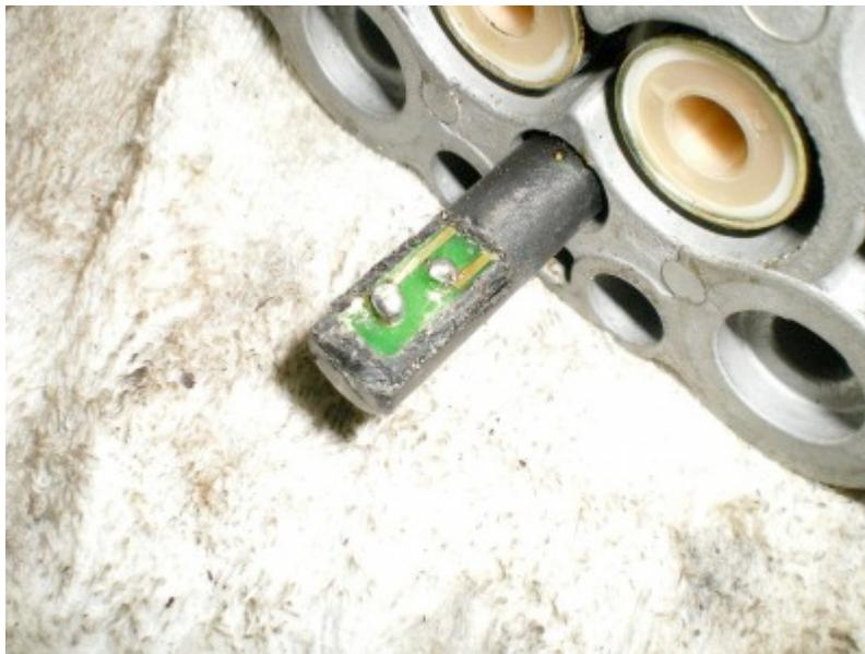
I filed off some of the excess solder to make sure it would not contact the metal when I put the two halves back together. I then coated my work with some liquid electrical tape to seal up the connections. Three coats of it to be exact.
