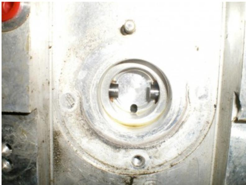
Here is what activates those two pins. As the motor spins, this bearing rides against the pins. You can kind of see how the bearing is offset of center.
