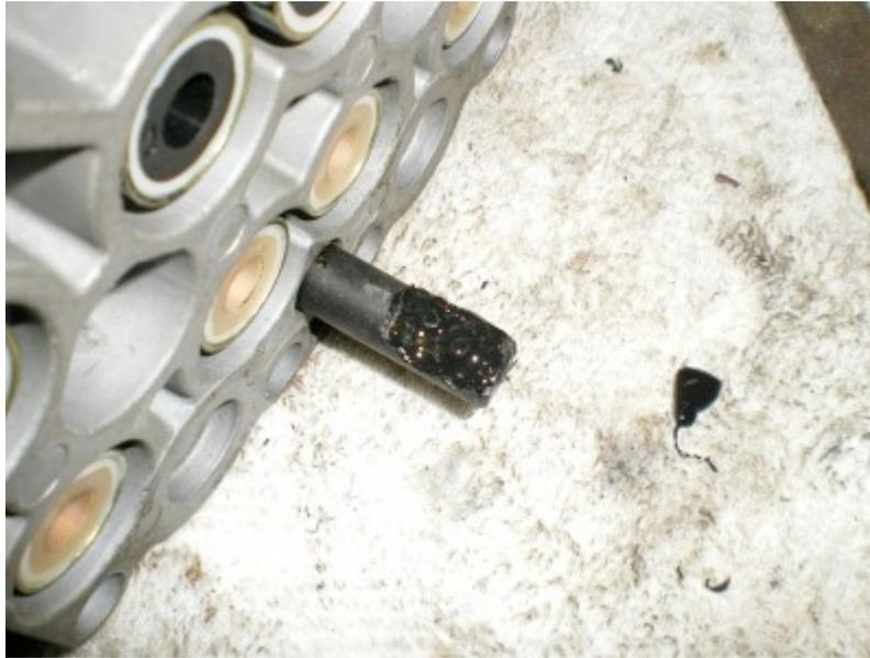
I put all the pieces back together and put the trusty ohm meter back on it. I found the most sensitive part was when tapping the actual black plastic of the shuttle valve in the center when conducting my testing early. Now with the connections "upgraded" i could hit the thing with a hammer and my readings would not change. There was a good solid connection that shouldn't jar loose when hitting even a pot hole!
