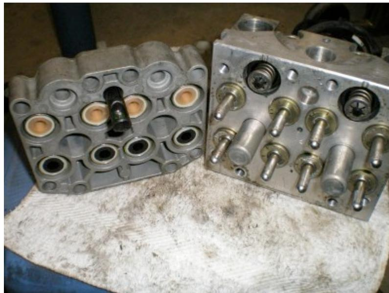
On the \*lower\* portion of the thin half of the case you will see a black plastic rod sticking out. It's obvious. This is where the shuttle valve connects to the circuit boards of the modulator.
