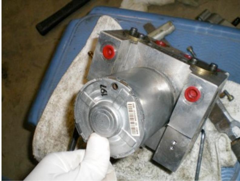
Here is what it looks like under the motor, those two pins work as mini brake pedals, you push one in and it develops line out pressure on its respective half of the modulator.
