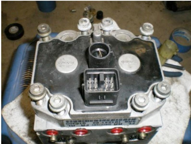
You might have to lightly pry the two halves apart and you will see the inner workings of the solenoids and valves that control your brakes and wheel spin for both abs and TT4. These silver rods move in and out in order to control which wheels receive the hydraulic pressure in the caliper. Don't worry there is nothing loose inside here that can fall out or move on its own.
