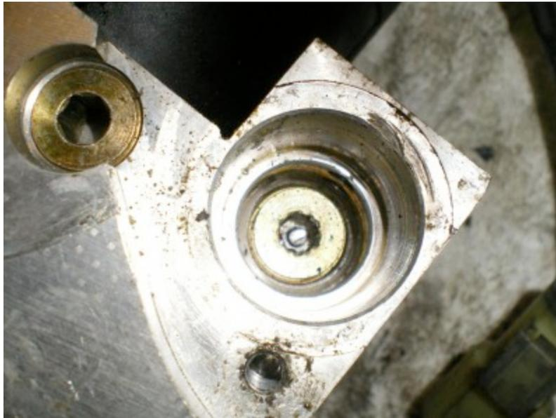
Back on track this left me with a problem in the connector. This is where the internet did its purpose and allowed me to find another Land Rover owner who did this same process. There are eight bolts holding the two halves of the modulator assembly together. Remove these eight bolts and make sure your shuttle valve is not connected.
