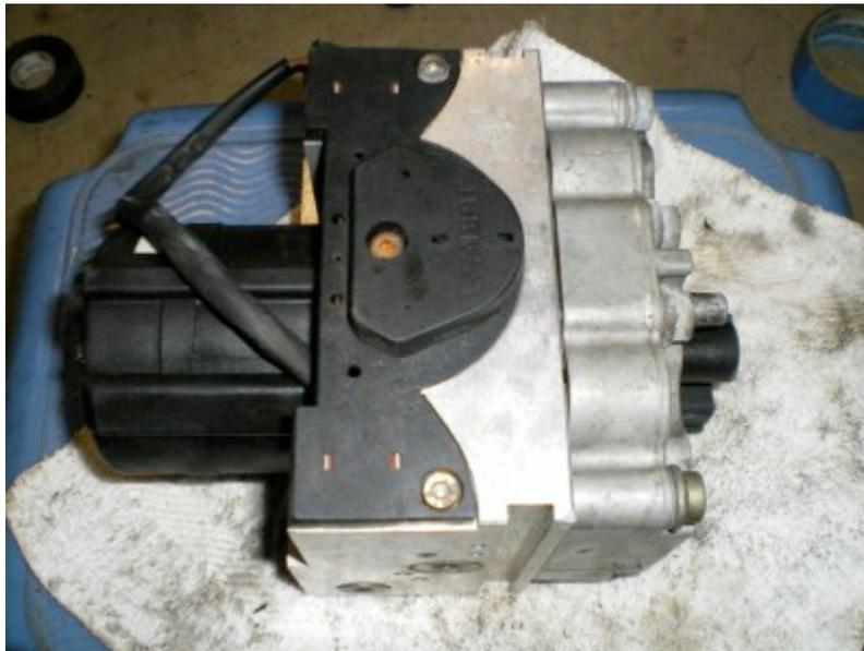
I took the side of my ratchet/socket wrench and tapped on that box with the ohm meter hooked to the pins. There in lies my problem, I would tap it and the connection would open up allowing current to pass through, tap again and it's gone, and so on.
