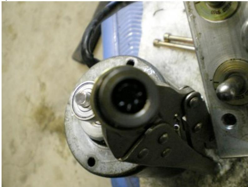
These are some other plugs that I could unscrew. Some of the were not interested in coming out like.....the plugs where the pins of the shuttle valve are activated, the center big plug/ screw on the side, and the small ones between the big holes under the shuttle valve.
