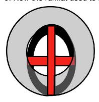
10. Put a rod like shown in the picture thru the runflat and remove the last compressor you set. (Take dish soap to make the rod sliding through).
