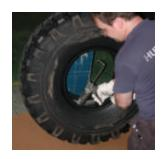
Raise the VFI with two small blocks (not included) to ease the manual VFI compression tool (Z) strap around it. Wrap the strap around the diameter of the tire and thread the end through the fastener on the compression tool, taking up as much slack as possible. (Refer to Compression Tool Strap Threading, page 15)
