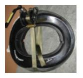
Crank until the two sides are within three inches of touching. Remove the crank handle from the compression tool.
