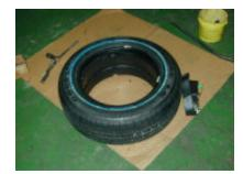
2. Insert the strap (in the direction that will enable the ratchet to compress properly) over top of the runflat and feed past the other head.
