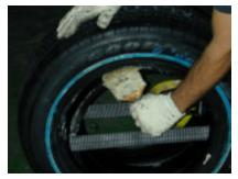
8. Center the runflat with the strap facing 3 & 9 O'clock as shown. Make sure the runflat is press as far to the bottom as possible.
