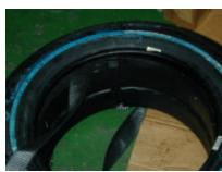
Roll the tire and runflat around so the portion of the strap you are feeding through can be pulled over top of the runflat.
