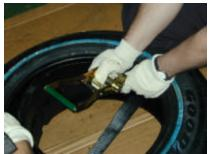
6. Feed the strap end through the ratchet hub barrel and pull tight. Ratchet the strap for about one turn.
