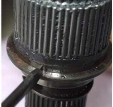
This shows the bearings in place on the mainshaft. During assembly they are held in place by petroleum jelly.
