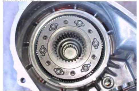
The outer annulus and inner assembly with the planet gears are now exposed, once the shifter mechanism is removed.
