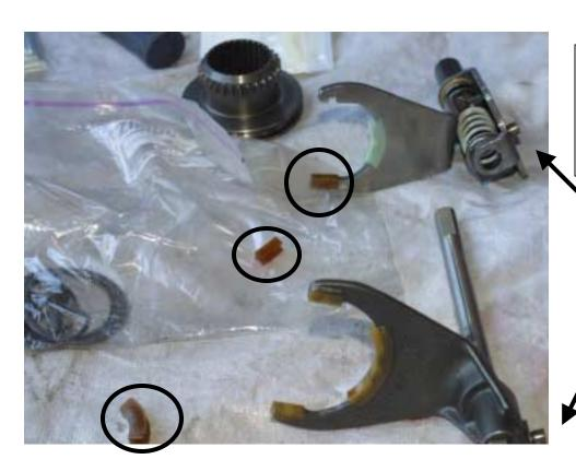
Each shifter fork has three plastic pads. The arrow identifies the pin At this time, only the input gear assembly with the planetary gear assembly remains in the front case halves.
