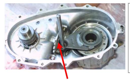
The upper slot in the sector plate for the mode arm pin is just visible. To remove the arms, you must manipulate the operating lever while twisting the arm to dislodge the pin. Once unengaged, the arm can slide away from the rail.
