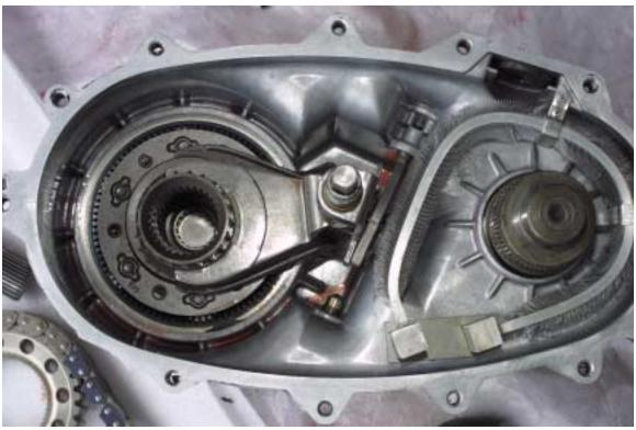
This is the civilian transfer case with the cooling loop only found in the "driven gear" half of the front case.
