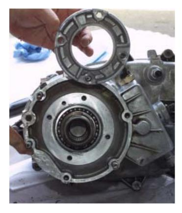
By removing a snap ring, the input gear and planetary assembly can be removed from the case. Several snap rings will hold this unit together.
