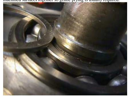
The rear bearing extends beyond the housing by 0.124 inch. This is proper seating of this bearing.
