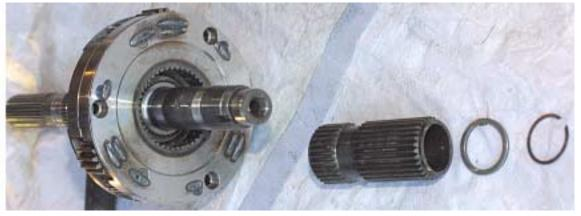
Remove the snap ring immediately prior to the differential assembly. The assembly can be removed from the mainshaft. Note: perform this is a clean flat work area for individual bearings will fall out upon separating the two components.
