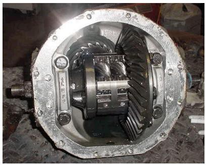
Torsen Differential with Ring Cover removed
