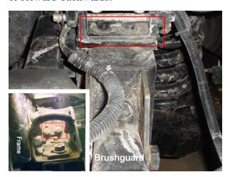
Figure #7 Illustrates the forward view of the alignment bolts and the insert on the lower left shows the corresponding nuts that are located under the truck in the center of the front hold down brackets.
