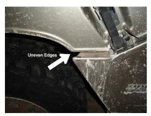
Figure #3 is a side view of the truck that reveals that the imaginary line arc from body to hood wheel well is out of alignment. The gap may also not be uniform along these surfaces.
