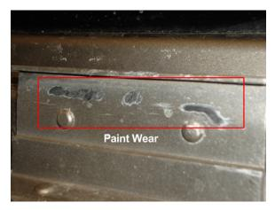
Figure #2 shows abnormal paint wear on the firewall from the hood impacting it while moving rearward during hard offroading.
