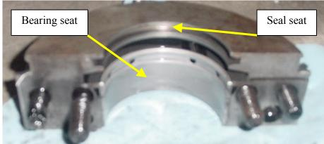
Rear Main Bearing Cap (seal removed)
