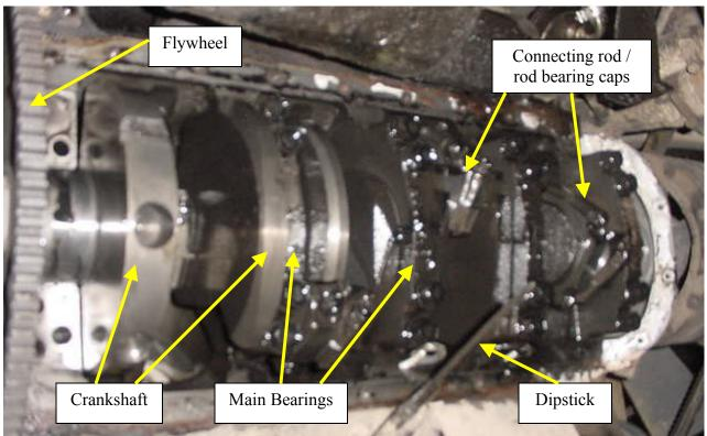
Crankcase with oil pan removed (oil pump / rear-main not installed)
