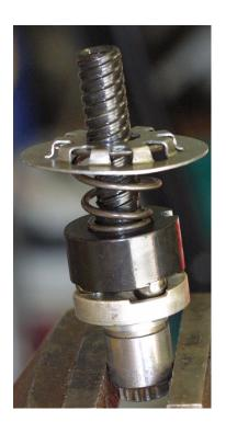
The trust screw and the actuator shaft have between them three steel balls. These balls fit into eccentric indents. This will provide a one-way movement to the thrust screw when under compression. This is why when changing brake pads you must both compress and rotate the piston to retract it.
