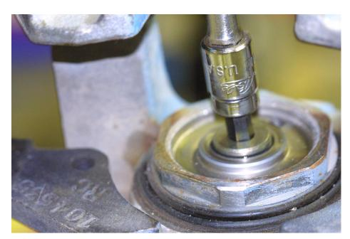
5. To remove the piston, I used the Breggin tool with a 3/8 extension and ratchet. <a href="http://www.bluehummer.com/rebrcacoto.html">http://www.bluehummer.com/rebrcacoto.html</a> You then turn the piston counterclockwise. This can remove the piston about 2/3 of the total distance quickly. Then, you must remove this tool and use large channel locks on the same flat surface to totally unscrew the piston. Protect the surface from scratching.
