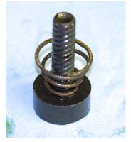
10. With the thrust screw removed, remove the thrust screw centering pin plug, spaced and finally with your finger inside the piston cylinder push the centering pin out. Discard O-ring.
