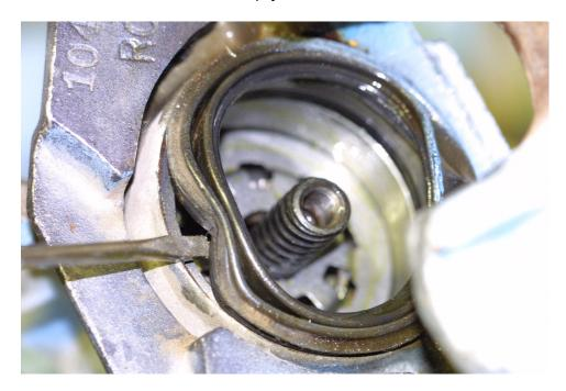
8. To remove the thrust screw-retaining ring (spring), it is easiest if you have the correct tools. I would recommend using the **SK HAND TOOLS** - **HOOK & PICK SET, 90353.** Either be very careful to not touch the inner piston cylinder surface or wrap the tools with a thin layer of electrical
