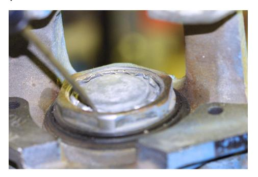
4. Remove the piston retaining screw with a hex socket. This screw has a rubber O-ring seal and a beveled shaped.
