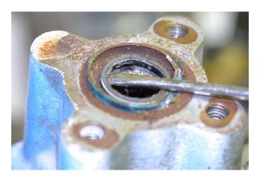
14. Remove the caliper piston seal with a SK hook and discard.
