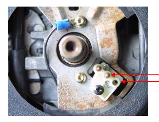
This is the modified brush mechanism. The arrows show the new location of the pin to the middle position.
