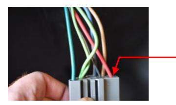
Insert the paper clip here to test the circuit.
