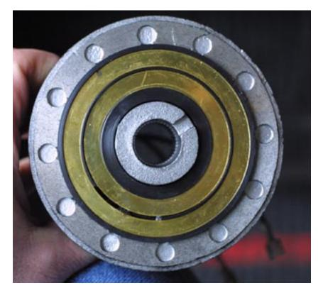
The new pin location will now align with the Momo adapter horn contact rings.
