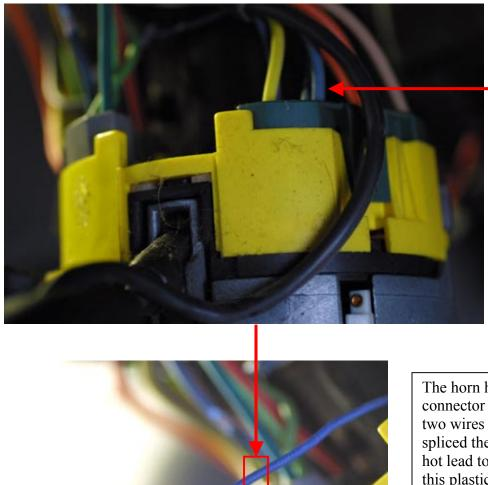
The upper multiconnector has the horn hot wire. The horn will sound if this wire is touched to ground.
